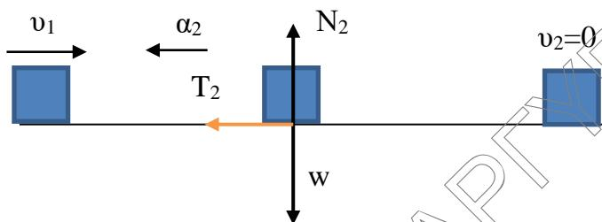
$$\sum F_y = 0 \Rightarrow N_2 - W = 0 \Rightarrow N_2 = 40 \text{ N} \text{ και } T_2 = \mu N_2 \Rightarrow T_2 = 20 \text{ N}$$
